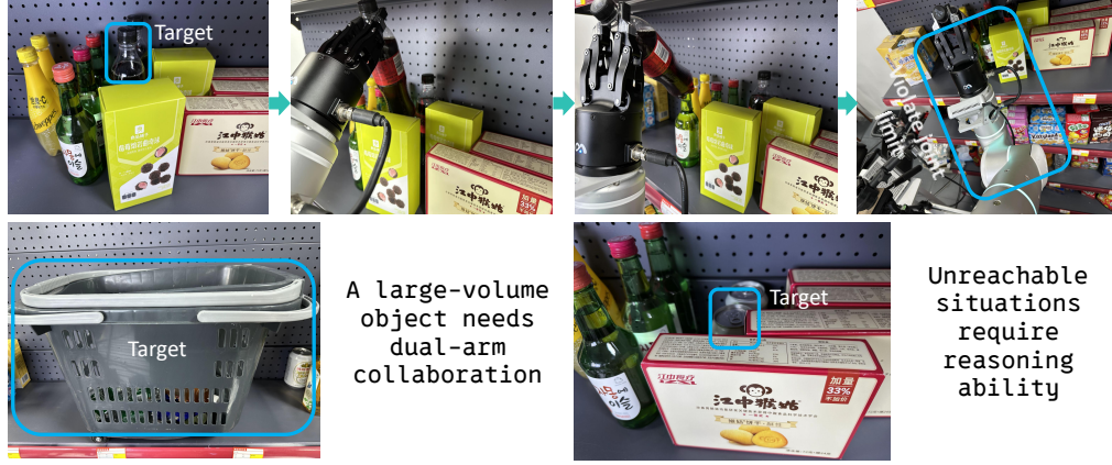
Figure 18: Illustration of Limitations. (Top row) Actions exceeding joint limits due to an attempted approach from above. (Bottom row, left) A large-volume object demonstrating the need for dual-arm manipulation. (Bottom row, right) A completely occluded and initially unreachable target, necessitating a multi-step reasoning process involving moving the obstacle, fetching the target, and subsequently returning the obstacle to its original position.
